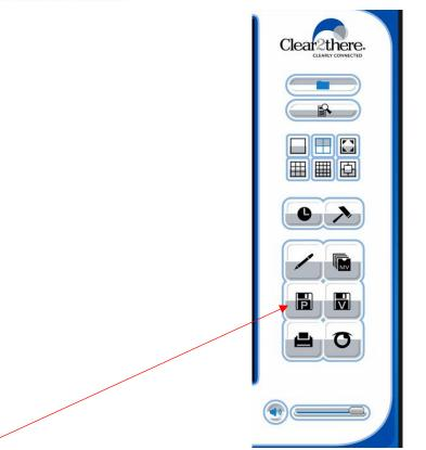
b. **Disc icon with P** is to save an image of the footage into a database. It will bring up a pop up that allows you to save an image file of whichever camera is selected. Press **SAVE** to save the image selected.
